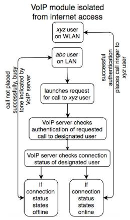
Fig. 7. Flowchart of call request from user *abc* to user xyz in module.
