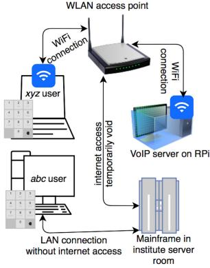
Fig. 6. Pictorial representation of implemented VoIP module.
