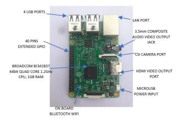
Fig. 2. Top view of Raspberry Pi 3 model B.
