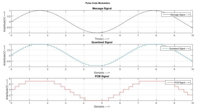
Fig. 3. Pulse code modulated sine wave with 256 quantization levels.
