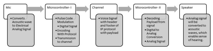
Fig. 1. Block Diagram of a basic VoIP system.
